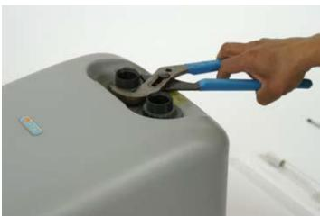
Use tongue and groove pliers or similar to loosen plastic nuts holding the housing in place. It is not necessary to grip nuts tightly, a loose grip will help prevent scarring of plastic. If desired, a piece of duct tape may be used to cover the teeth of the tongue and groove pliers to prevent scarring of the plastic nuts.
