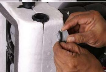
Remove plug and o-ring from ring nut.
