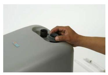
Once loosened, manually remove the plastic nuts.
