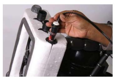
Insert Heater into heat exchanger until o-ring seats into outlet lip. If you encounter resistance while inserting the Heater, gently turn the Heater and apply very slight force.
