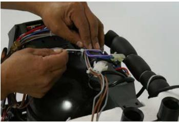
Use cable tie to fasten wiring harness to support strut.
