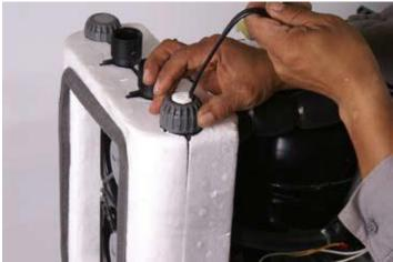
Use tongue and groove pliers or similar to ensure there is no leak.
