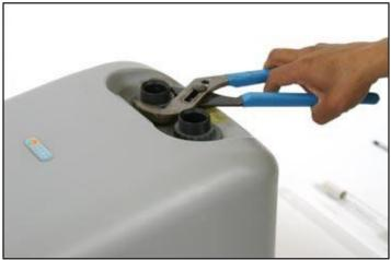
Use tongue and groove pliers or similar to loosen plastic nuts holding the housing in place. It is not necessary to grip nuts tightly, a loose grip will help prevent scarring of plastic. If desired, a piece of duct tape may be used to cover the teeth of the channel lock pliers to prevent scarring of the plastic nuts.
