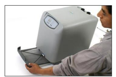
Remove air filter from chiller housing.
